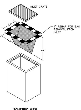
Maximum Drainage Area = 1/2 Acre Inlet Protection is not required for inlet tributary to sediment basin or trap. DO NOT USE ON MAJOR PAVED ROADWAYS WHERE PONDING MAY CAUSE TRAFFIC HAZARDS
