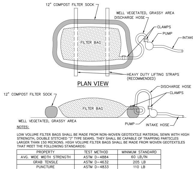
MULLEN BURST ASTM D-3786 350 PSI ASTM D-4355 UV RESISTANCE 70% AOS % RETAINED ASTM D-4751 80 SIEVE A SUITABLE MEANS OF ACCESSING THE BAG WITH MACHINERY REQUIRED FOR DISPOSAL PURPOSES SHALL BE PROVIDED. FILTER BAGS SHALL BE REPLACED WHEN THEY BECOME 1/2 FULL OF SEDIMENT. SPARE BAGS SHALL BE KEPT AVAILABLE FOR REPLACEMENT OF THOSE THAT HAVE FAILED OR ARE FILLED. BAGS SHALL BE PLACED ON STRAPS TO FACILITATE REMOVAL UNLESS BAGS COME WITH LIFTING STRAPS ALREADY ATTACHED.
