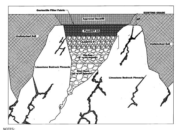
1. THE REPAIRS OUTLINED BELOW ARE GENERAL GUIDELINES AND EACH SINKHOLE OCCURRENCE SHOULD BE THOROUGHLY REVIEWED BY THE GEOTECHNICAL ENGINEER OF RECORD FOR AN APPROPRIATE REMEDIATION PLAN:
